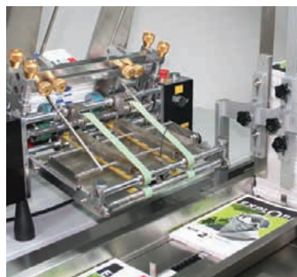
Friction feeder for feeding single sheet paper
